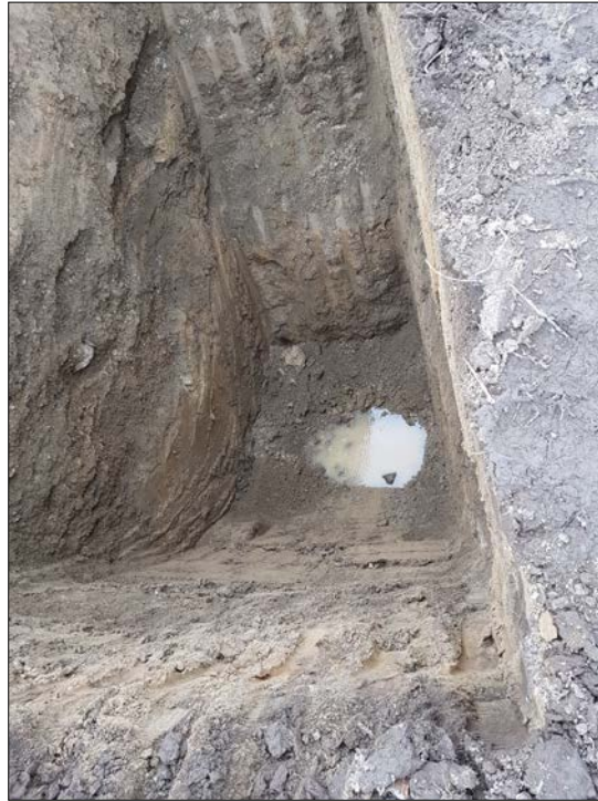
Photo showing water collected in Test Pit A after 1.5 hours.
