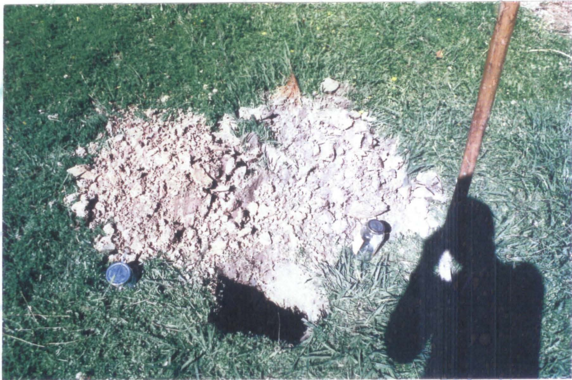
Photo 2 - Test hole showing subsurface materials of topsoil and silty loam
