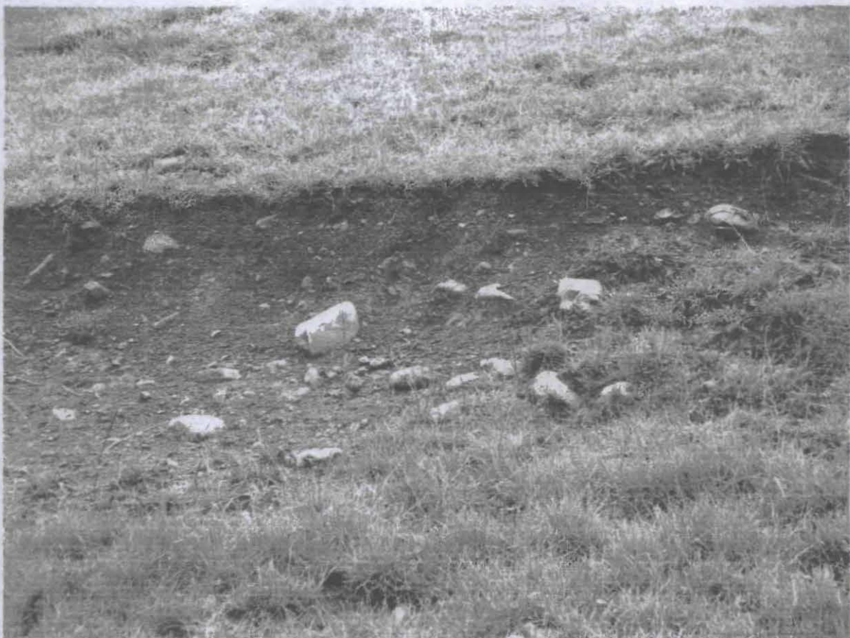
Photo 2: Exposure of site soils - gravel boulders in clay matrix.
