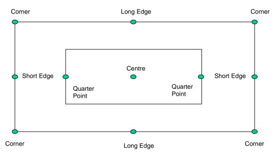
The values given for spring stiffnesses are estimated mean values but it must be understood that the values could vary across the site. Therefore, we recommend that a sensitivity analysis be performed during raft design, by alternatively halving and doubling individual stiffness values. Furthermore, the
