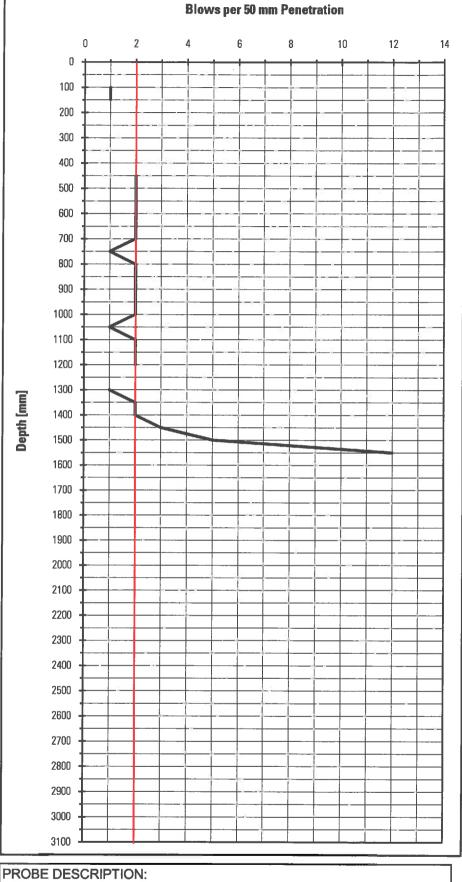
9 kg Hammer falling half a metre to a steel anvil, driving a 16 mm diameter rod fitted with a 20 mm diameter cone.
